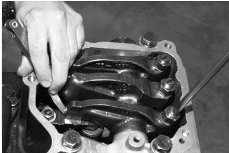
Fig 3-12. Adjusting valves.
