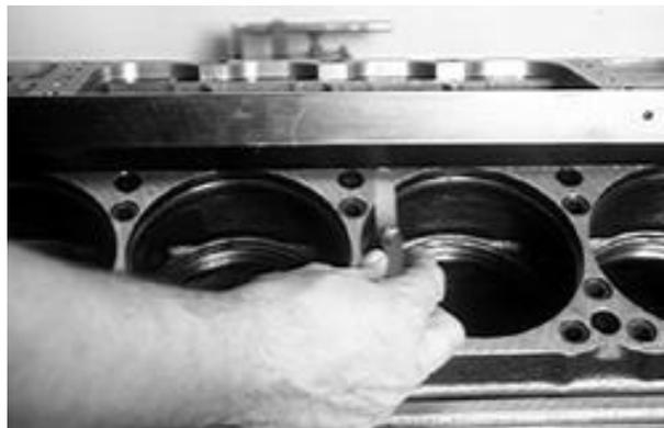
Fig 5-2. Checking cylinder block warpage.
