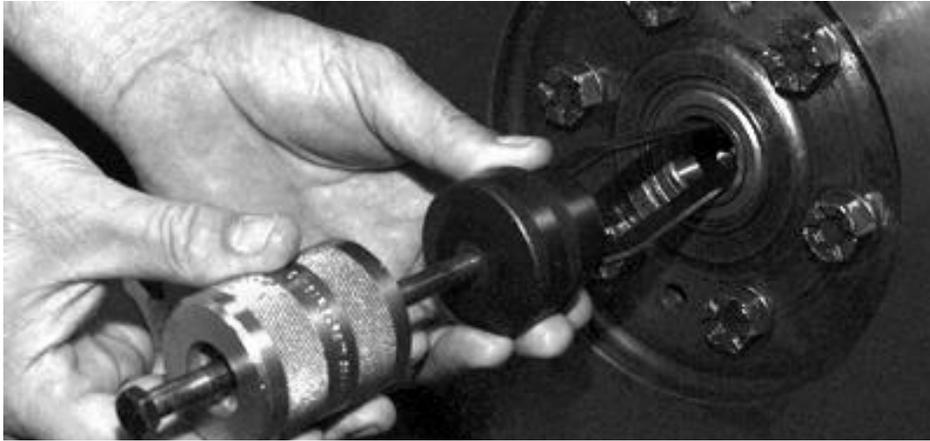
Fig 4-12. Removing the clutch pilot bearing.
