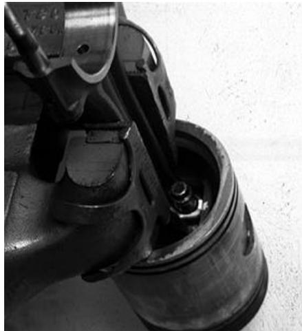
Fig 5-16. Secure piston in vise.
