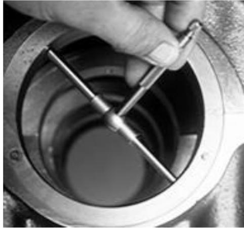
Fig 5-13. Measuring the crankshaft bore with a telescopic gage.
