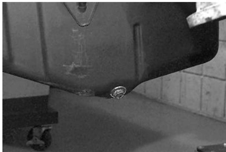
Fig 4-2. Drain the engine.
