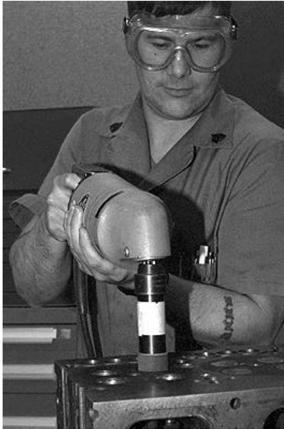
Fig 5-27. Grinding valve seats.
