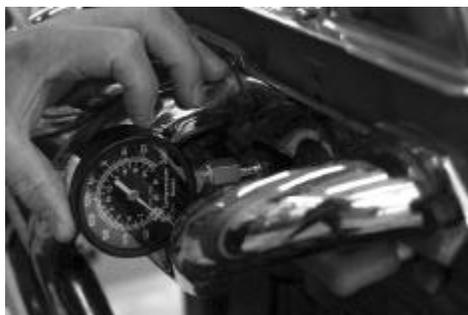
Fig 3-1. Inserting compression gage into spark plug hole.
