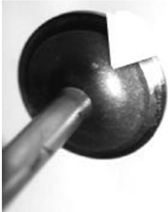
Fig 3-11. Example of valve wear.
