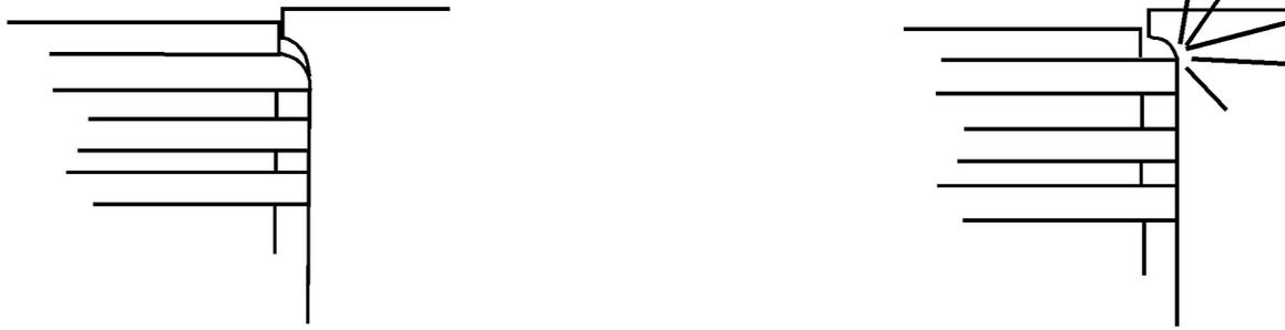
Fig 4-7. Result of installing new piston rings with ridges at the top of the cylinder.
