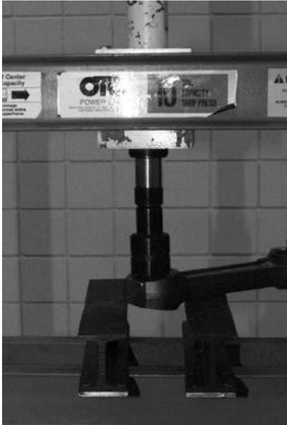
Fig 5-23. Installing piston pin bushings.
