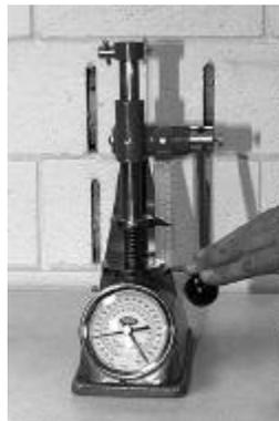
Fig 5-31. Checking valve spring pressure.
