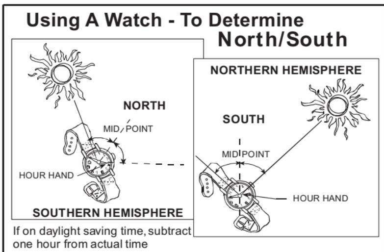
Figure II-2. Direction Using a Watch
