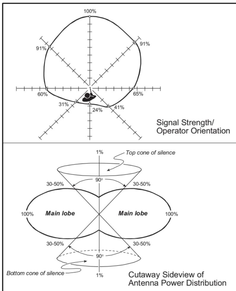
Figure III-1. Radio Transmission Characteristics
